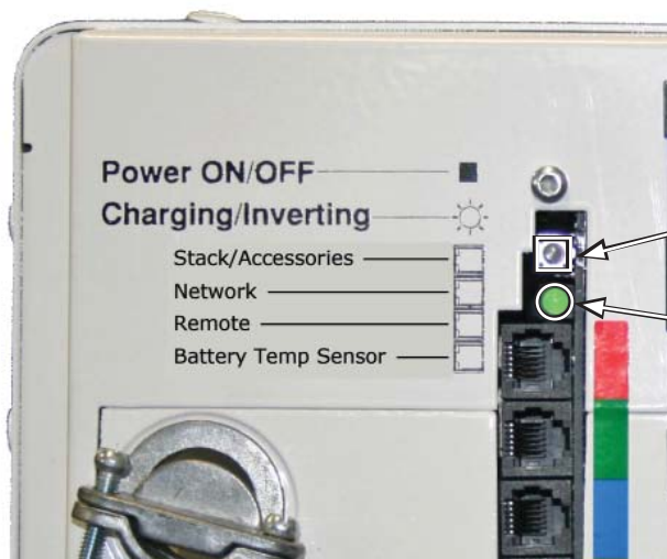
Figure 4-1, Performing an Inverter Reset
