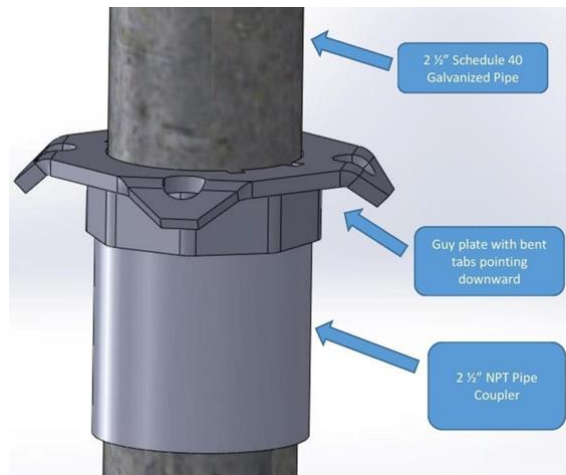
Figure 5.2 – Guy plate orientation detail
