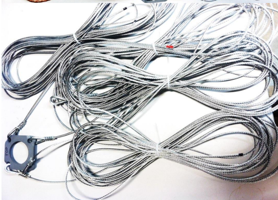
Figure 2.1 – 63' EconoTower Hardware Kit contents (tower base angles not shown). Top left: hardware; bottom left: guy plate assembly (1 of 3 with the 63' EconoTower). NOTE: red tape marks the rear guy cable of each guy plate assembly. The rear guy cable has an eye thimble swaged onto it for attachment to the gin pole. Guy plates are labeled BOTTOM, MIDDLE and TOP ; top right: gin pole guy ropes, front guy rope, flex conduit, grease and brush.
