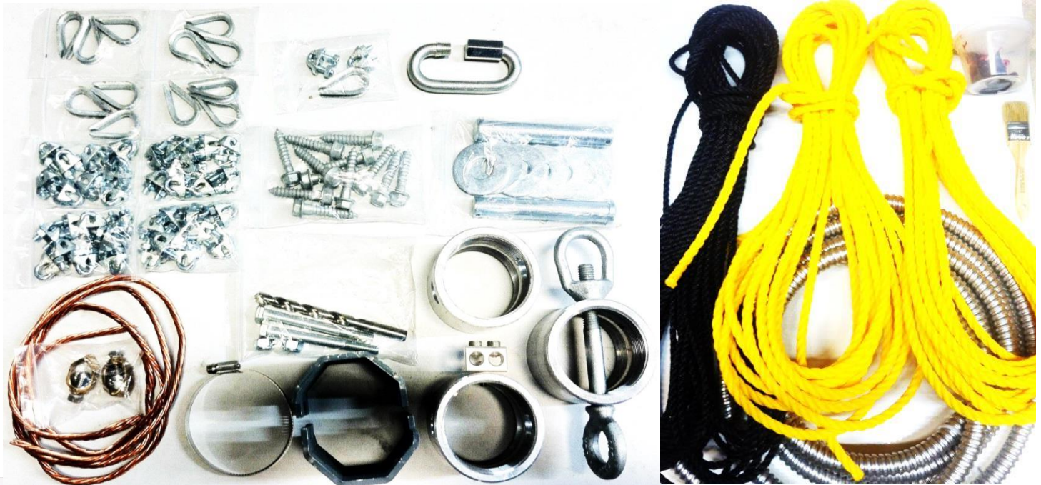
Figure 2.1 – 63' EconoTower Hardware Kit contents (tower base angles not shown). Top left: hardware; bottom left: guy plate assembly (1 of 3 with the 63' EconoTower). NOTE: red tape marks the rear guy cable of each guy plate assembly. The rear guy cable has an eye thimble swaged onto it for attachment to the gin pole. Guy plates are labeled BOTTOM, MIDDLE and TOP ; top right: gin pole guy ropes, front guy rope, flex conduit, grease and brush.
