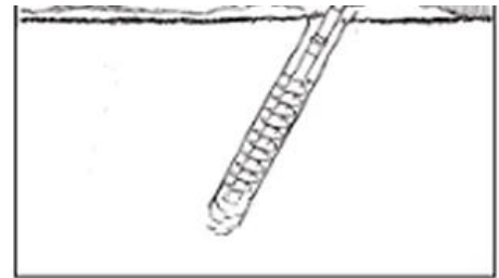
Figure 4.3 – 8" auger at 45-60 degrees from horizontal
