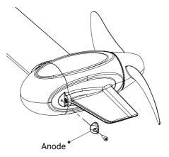
Figure 10-1 Replace Pod Drive1.0 Evo anode
