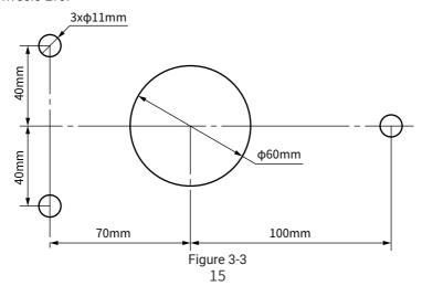
**Step 2:** Hold the pod motor and insert its three bolts (Pod Drive 1.0 & 3.0 are M8, Pod Drive 6.0 Evo is M10) and supporting tube into the holes from below the hull bottom. Then lock the each bolt from inside the boat by a plain washer and a nut (Figure 3-4).
