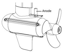
Figure 10-2 Replace Pod Drive6.0 Evo anode
