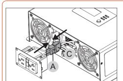
Attach the two connectors together  $A \rightarrow \leftarrow C$ .
