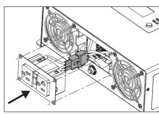
Mount the GFCI device onto the inverter unit.
