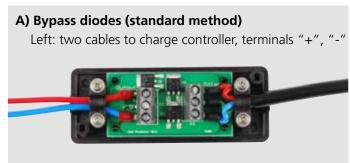
With this hookup, the cells are protected with 2 bypass diodes against the hot spot effect.
