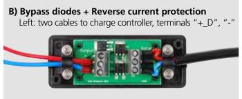
With this hookup, the cells are protected with 2 bypass diodes against the hot spot effect and the additional blocking diode protects against reverse current back into the module. By damage to a module or cable by several modules in parallel operation, an influence can be prevented on the other modules with the use of the blocking diode.
