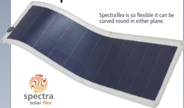
The Spectraflex is a solar panel made from a spectrum splitting amorphous silicon cell design that converts very low levels of light to useable solar energy. Unlike other types of amorphous silicon technology the Spectraflex is very stable over many years where others degrade rapidly soon after deployment. Bypass diodes are connected across each cell so the panel is also shadow tolerant.
