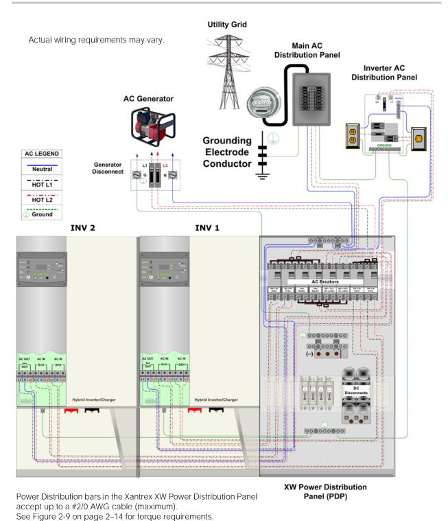
Figure 2-29 AC Wiring for Dual-Inverter Systems
