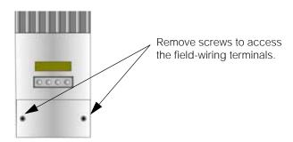
Figure 4-2 Removing the Wiring Compartment Cover
