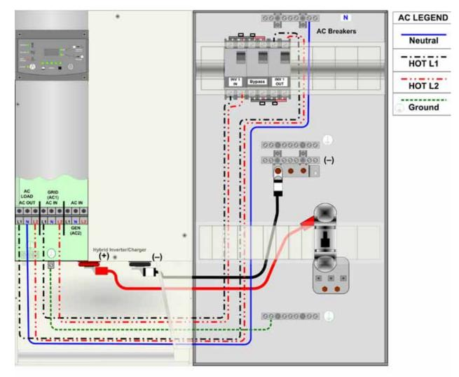
Power Distribution bars in the Xantrex XW Power Distribution Panel accept up to a #2/0 AWG cable (maximum). See Figure 2-9 on page 2–14 for torque requirements.
