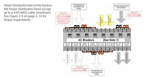
Figure 2-28 Dual Inverter AC Breaker Arrangement and Wiring Enlargement with Multiple AC Input Sources
