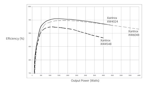
Figure A-8 Grid-tie Sell Mode Efficiency (Typical)
