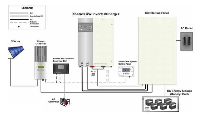
Figure 3-1 Network-Managed Power System
