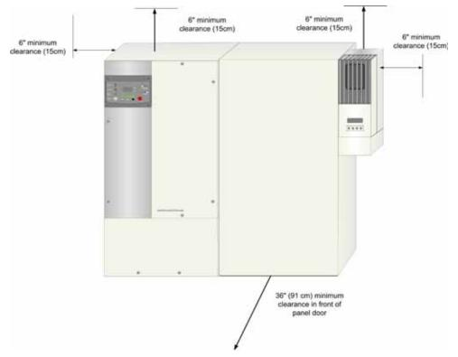
Figure 2-3 Clearance Requirements
