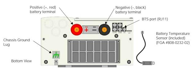
Figure 2-11 Xantrex XW Inverter/Charger DC Connections
