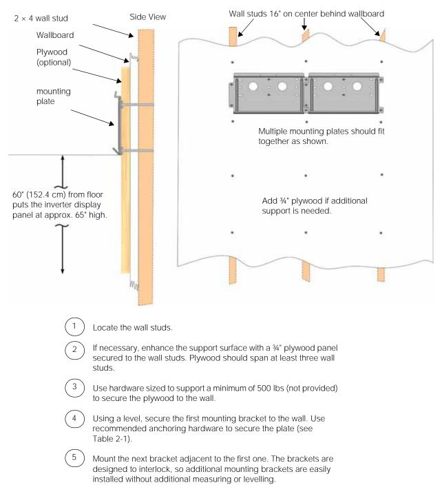
Figure 2-5 Mounting the Bracket for the Xantrex XW Inverter/Charger or Distribution Panel
