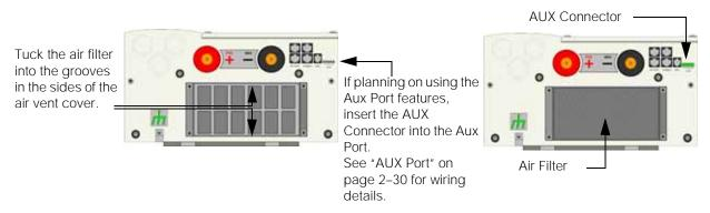
Figure 2-1 Air Filter and AUX Connector Installation
