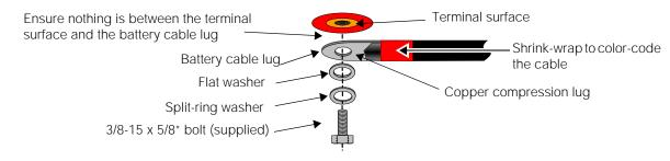
Figure 2-12 Battery Cable Connection
