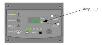
Figure 2-25 Checking Charging Operation
