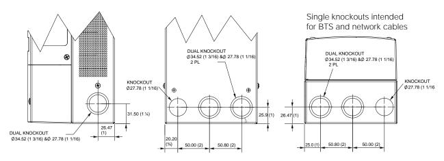
Figure 4-4 Knockout Dimensions
