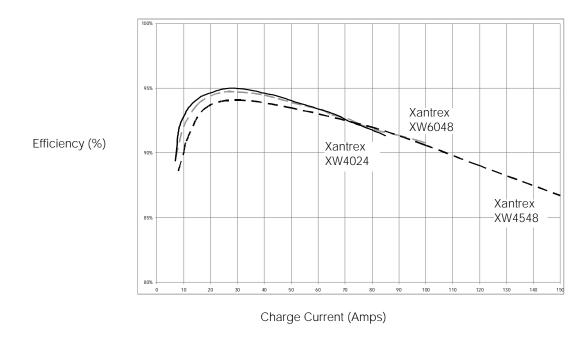
Figure A-6 Charging Efficiency (Typical)
