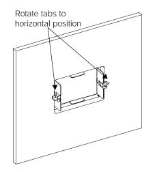
Figure 5-3 Securing the Mounting Plate
