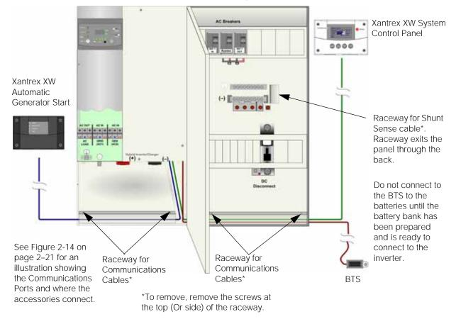
Figure 2-8 Routing Communications Cables
