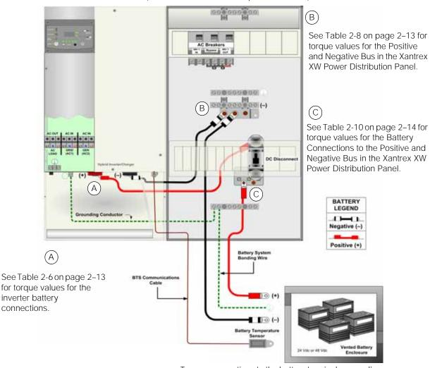
Torque connections to the battery terminals according to the battery manufacturer's recommendations.
