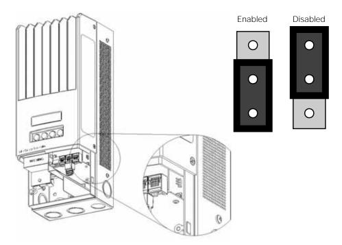
Figure 4-7 PV Negative Ground Jumper Location
