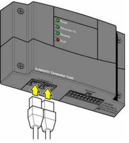
Figure 5-12 Connecting the Xantrex XW SCP
