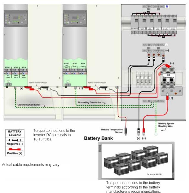
Figure 2-27 DC Connections to Dual Inverters
