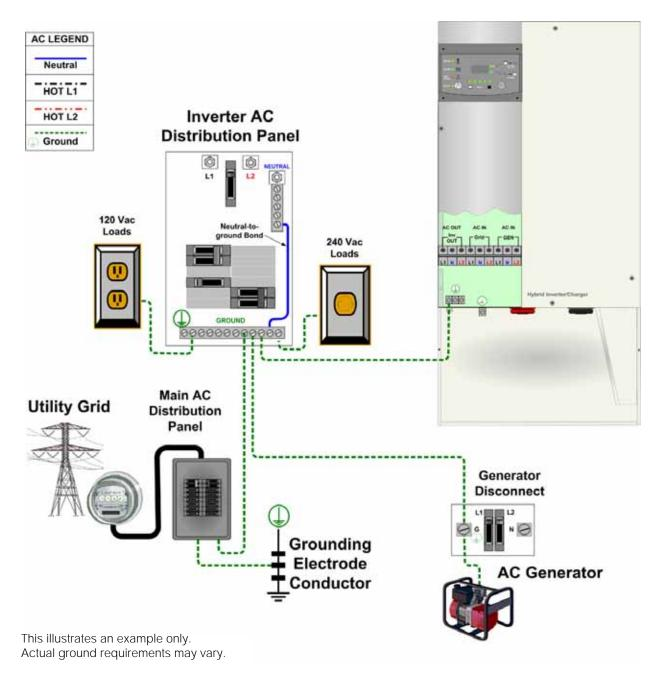
Figure C-3 Grounding the AC System
