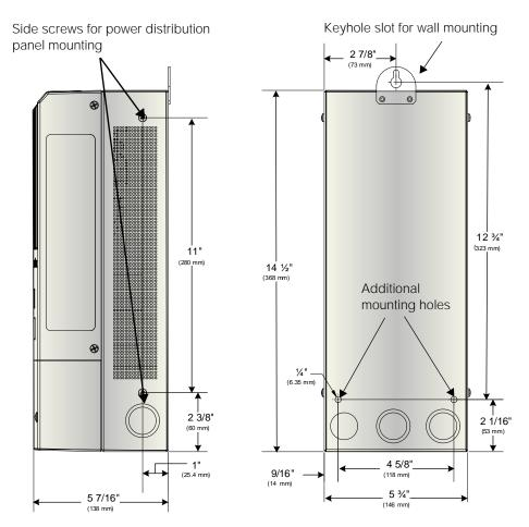
Figure 4-3 Dimensions and Knockout Locations
