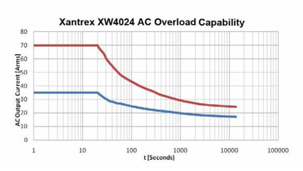
Figure A-3 Xantrex XW Series AC Overload Capability
