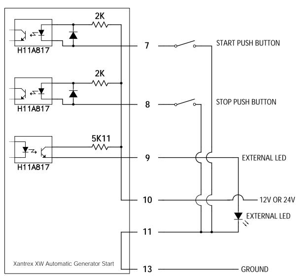
Figure 5-10 External ON/OFF Switch and LED Wiring Diagram
