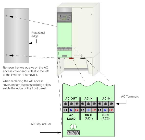
Figure 2-15 AC Terminal Block
