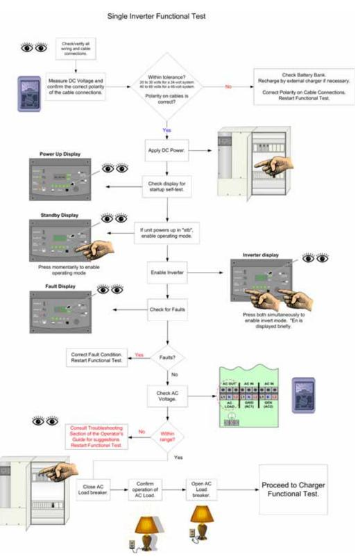
Figure 2-26 Functional Test for Single Inverter Systems
