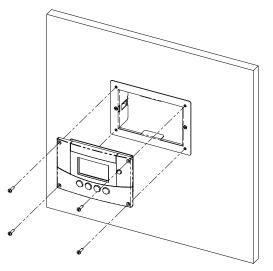
Figure 5-5 Securing the Xantrex XW System Control Panel
