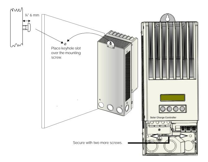
Figure 4-5 Mounting the Xantrex XW Solar Charge Controller
