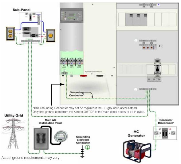
In an off-grid installation (i.e., where no utility grid is available), the generator can be connected to the breakers provided in the Xantrex XW Power Distribution Panel. No additional breaker is required. \* Depending on the location of the generator and local code requirements, the generator disconnect may be located in the power distribution panel.
