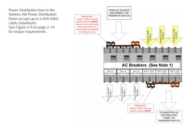
Figure 2-33 Triple-Inverter AC Breaker Arrangement and Wiring Enlargement with a Single AC Input Source
