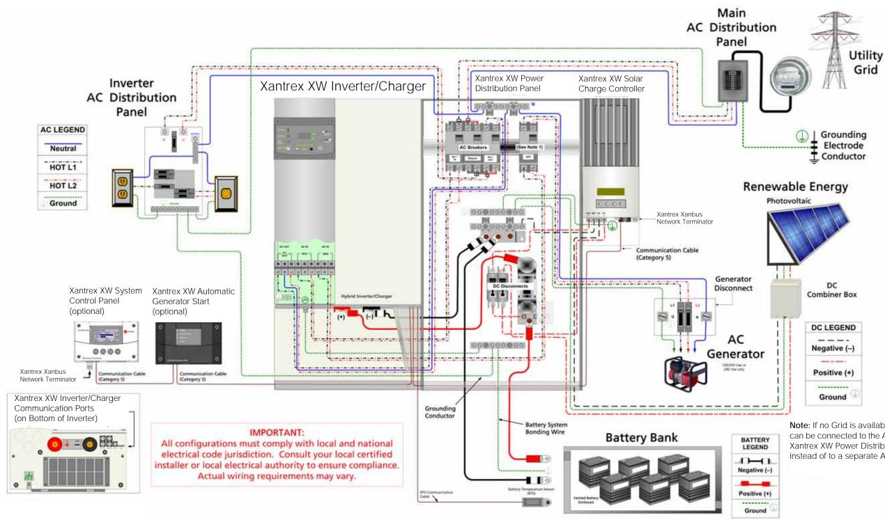
Figure B-3 Single-Inverter System Renewable Energy (Solar)
