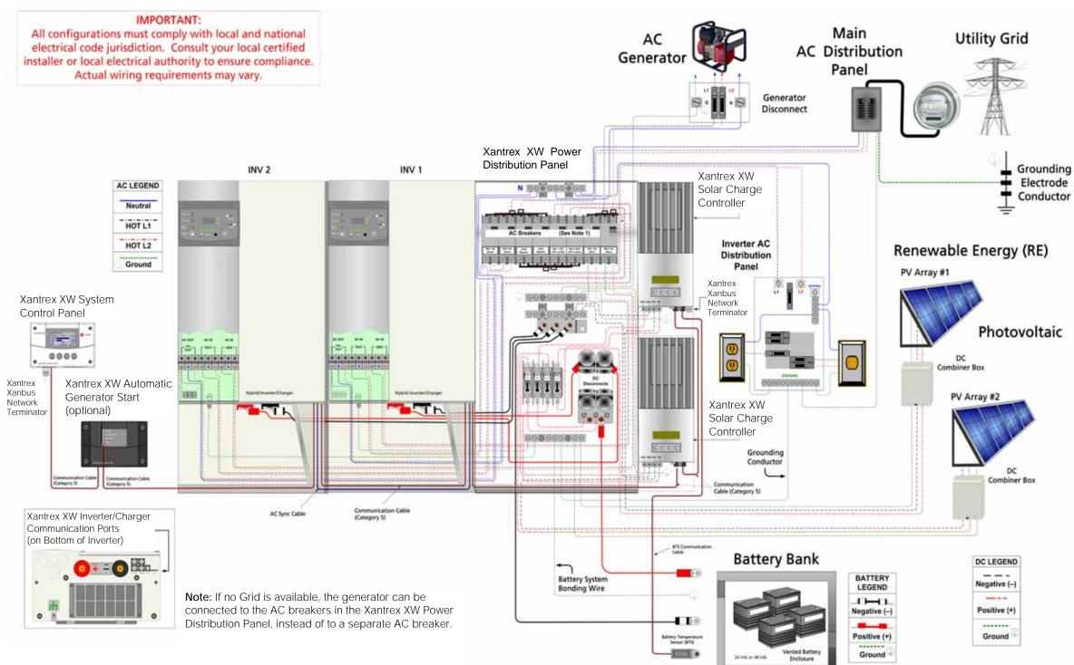
Figure B-5 Dual-Inverter System Renewable Energy (Solar)
