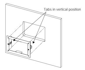
Figure 5-2 Inserting the Mounting Plate
