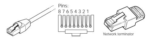
Figure 3-2 Xantrex Xanbus Cable, RJ45 Connector Pin Numbers and Network Terminators
