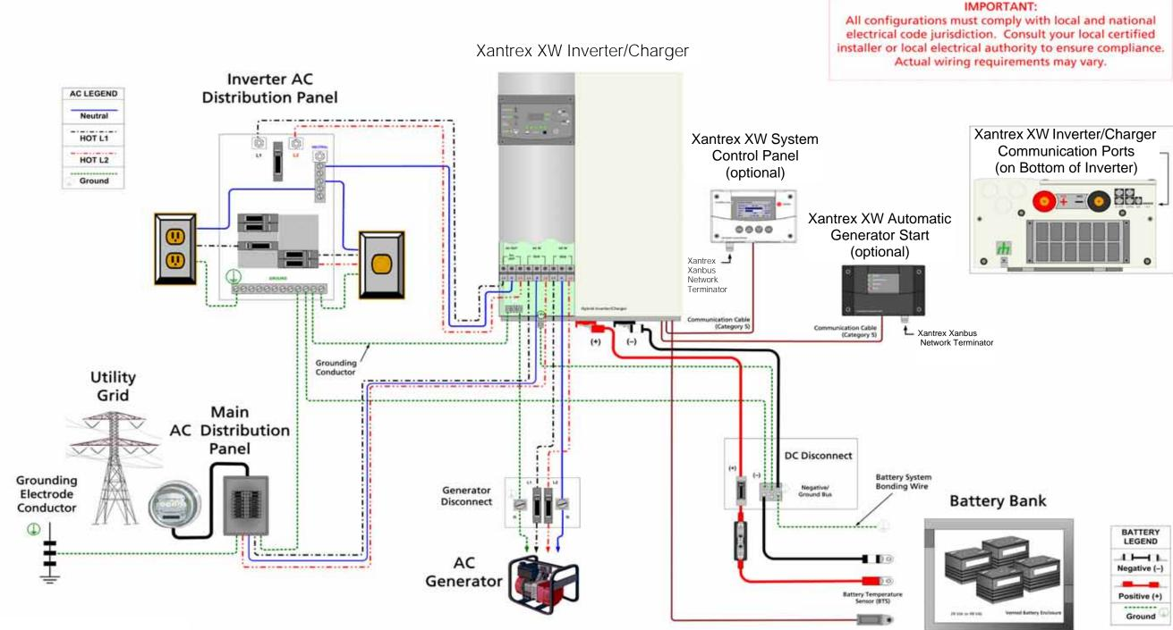
Figure B-1 Single-Inverter System (Backup Only) Without a Power Distribution Panel
