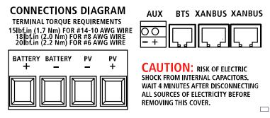
Figure 4-8 DC Connection Terminals
