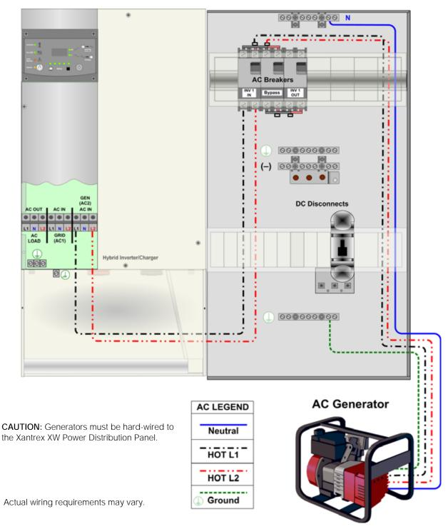
Figure 2-20 Generator Wiring Using a Xantrex XW Power Distribution Panel (Off Grid)
