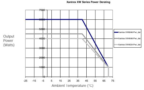
Figure A-4 Output Power Versus Ambient Temperature
