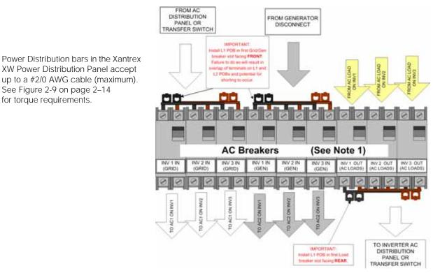
Figure 2-32 Triple-Inverter AC Breaker Arrangement and Wiring Enlargement with Dual AC Input Sources
