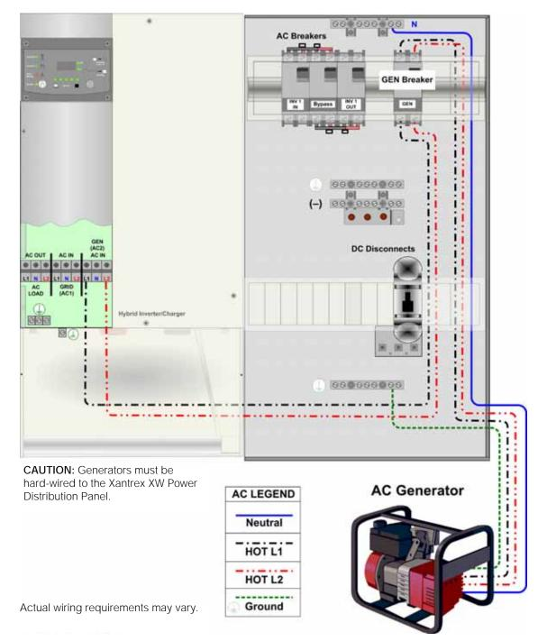
In an On-grid installation, the generator will require an additional AC breaker be installed in the Power Distribution Panel.
