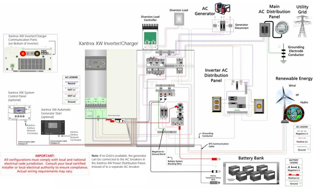
Figure B-4 Single-Inverter System Renewable Energy (Wind or Hydro)
