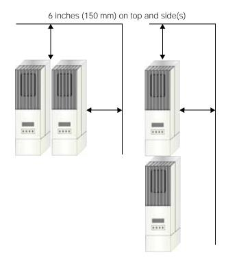
Figure 4-1 Minimum Clearance Requirements
