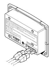
Figure 5-4 Connecting the Network Cables
