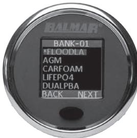
The currently selected battery type is noted with an asterisk (\*) in front of the name. The default is FLOODLA (see the chemistry table). If this is your chemistry and the installation is new, you may either re-select the chemistry, ensuring that the SG200 is starting fresh, or exit back to MENU and move to the next step.
