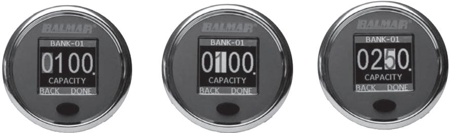
Once you select a chemistry, you must specify the capacity of the battery bank. This is the total design capacity of the entire bank, regardless of the battery's condition, or previously measured capacity. Typically the capacity is expressed as the 20-hour discharge rate. This may be written as something like "105Ah/20h" on the battery or battery documentation. If you cannot find
