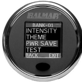
The Display menu allows for the configuration of the Display's colors, intensity and power usage.
