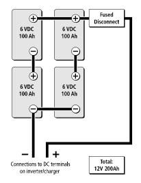
Figure 25 Batteries in Series-Parallel Connections
