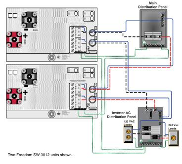
Figure 18 Series Stacking Using Two Freedom SW 3012s
