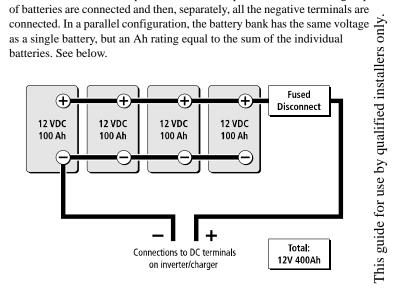
Figure 23 Batteries Connected in Parallel
