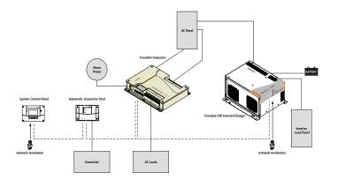
Figure 2 Typical Xanbus System Diagram
