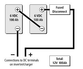
Figure 24 Batteries Connected in Series
