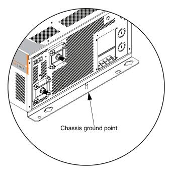
Figure 10 DC Wiring and DC Grounding
