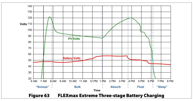
A new charge cycle is started any time the battery voltage decreases below the **Rebulk** set point for 90 seconds or more. (See page 36.) This usually occurs each night unless the batteries were maintained by another means. (If so, they may not need to be recharged).
