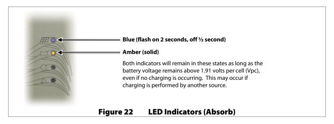
If the battery voltage drops below the **Absorb Voltage** set point (see page 36), the FLEXmax Extreme reverts back to the Bulk charge stage. The MATE3 displays **Bulk** as shown on page 25.
