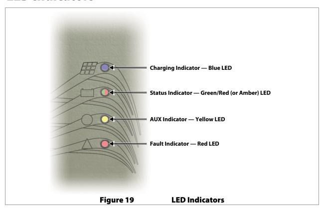
The FLEXmax Extreme charge controller has no graphical display. It is equipped with four LED indicators that show the charge controller's condition.
