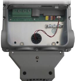
3. Insert the fan connector into the fan port in the controller's wiring box. It may be necessary to remove the rear plug and insert a bushing. (See illustration to the left; also see page 16.)
