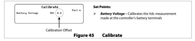
**NOTE**: Calibration does not change the actual voltage of the charge controller, only the reading of that voltage.
