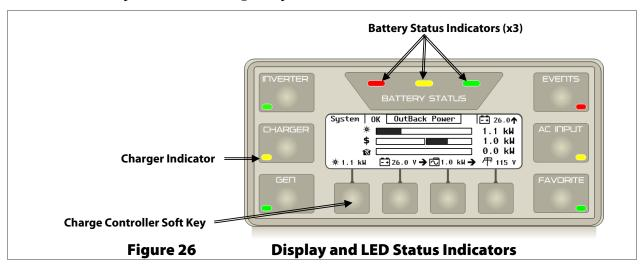
The MATE3 System Display and Controller is a display which allows the user to read the operating mode, measurements, and any status messages from the FLEXmax Extreme charge controller. It can also change the charge controller's settings when the default settings are not enough.
