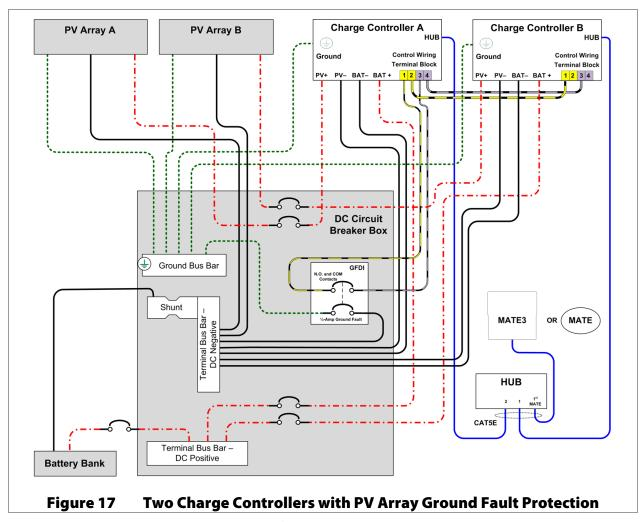
In Figure 17, a wire has been run from terminal 1 on Charge Controller A to one of the dedicated GFDI terminals. A wire has also been run from terminal 3 to the other side of the GFDI.
