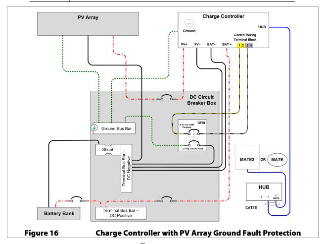
In Figure 16, a wire has been run from terminal 1 to one of the dedicated GFDI terminals. A wire has also been run from terminal 3 to the other side of the GFDI. As long as the GFDI remains closed, that pole of the GFDI will read as electrically continuous to the External Fault circuit.
