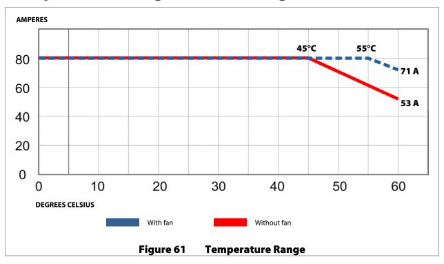
In standard installations, the FLEXmax Extreme can operate at its full 80-amp capacity at ambient temperatures up to 45°C (113°F). Above this temperature, its output is derated as shown in Figure 61. At 60°C (140°F), the output is derated to a maximum of 53 Adc. The controller is not rated for operation above this temperature.
