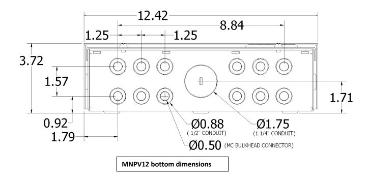
The following dimensioned drawings show the enclosure size and location of knockouts available on the MNPV12&16. Lightning arrestors may require a locknut on the outside in order to clear the lid.
