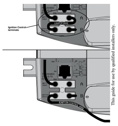
Figure 7 Exposed Ignition Control Terminals
