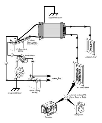
Figure 1 Typical Recreational Vehicle and Fleet Vehicle Installation
