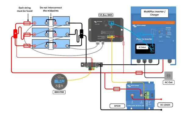
Our LFP batteries have integrated cell balancing and cell monitoring. Up to 5 batteries can be paralleled and up to four batteries can be series connected, so that a 48V battery bank of up to 1500Ah can be assembled. The cell balancing/monitoring cables can be daisy-chained and must be connected to a Battery Management System (BMS).
